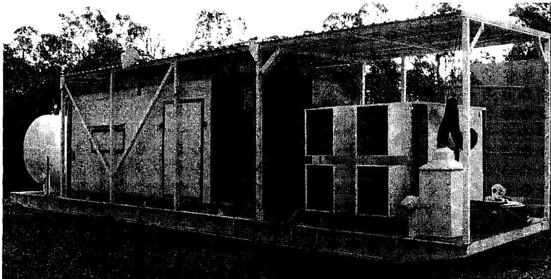
Figure 23: Austar 1800m 3 /hr Nitrogen Plant
