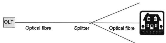
Several standards are available for FTTH networks. While the EPON standard has been widely deployed in Japan and Korea, the standard generally preferred in the USA, Europe and Australia is the ITU-T GPON (Gigabit Passive Optical Network).
