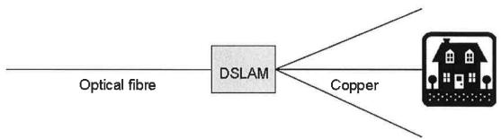
VDSL with FTTN has dedicated copper pairs for each customer. However, the optical backhaul link from the DSLAM is shared between all the customers served by that DSLAM (and potentially by other DSLAMs if the DSLAMs are daisy chained – which could be used, for example, where there are several DSLAM at a particular location sharing a single backhaul link, or several DSLAM closely located with each serving a small number of customers).
