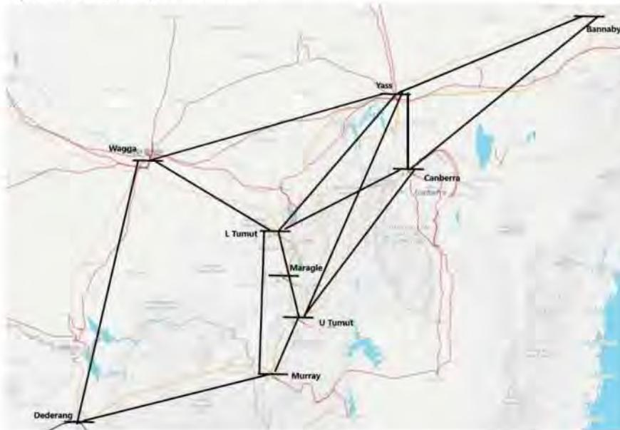
The TSIRP models the Canberra zone's flows and losses using DC load flow (DCLF) equations. DCLF is a simplified AC load flow which neglects reactive power flows. The model also captures the losses for the given lines through piecewise linear functions using the equivalent resistance of those lines.
