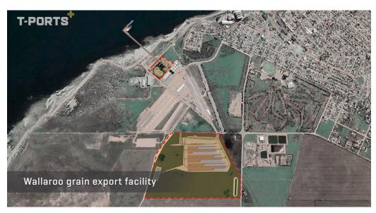
The Wallaroo Port infrastructure includes a rock armoured L-shaped causeway, at-port storage silos holding 20,500 tonnes, and upcountry bunker storage of 240,000 tonnes of grain.
