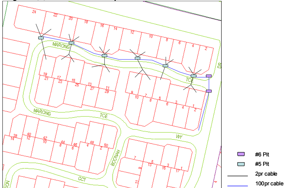
Figure 3(b): Illustrative example of conduit runs down two sides of the street
