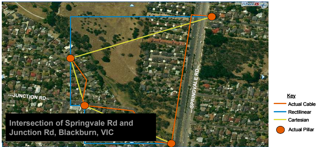
Figure 2: Example of Cartesian, Rectilinear and shortest feasible distances
