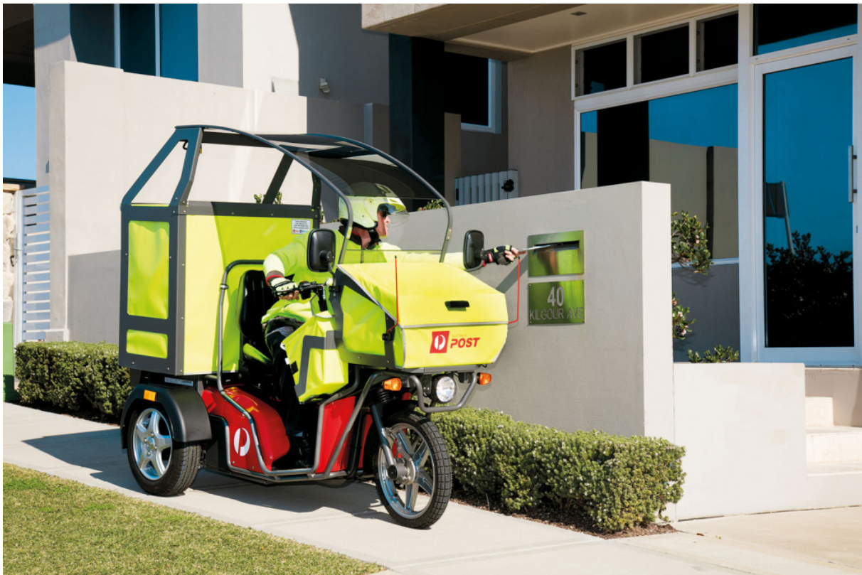
Above: Electric tricycle, capable of carrying up to 100 small parcels and 1200 letters
