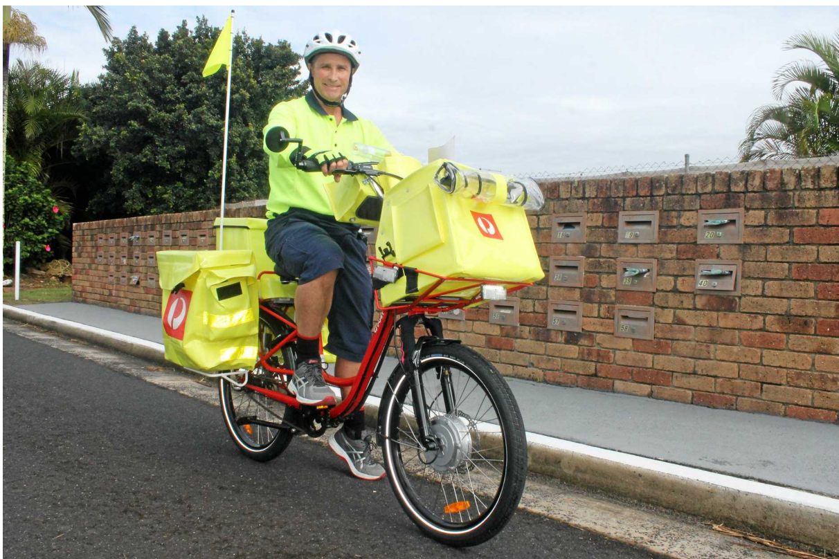
Above: electric-assisted pushbike, with same carrying capacity as petrol-powered delivery motorbike
