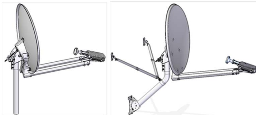
Figure 8.4: Satellite outdoor unit mounts (pole mount on the left, universal mount for walls, flat and angle roofs on the right) [Source: NBN Co, 2012]
