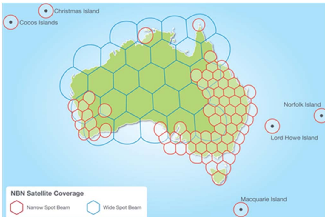
Figure 5.3: Proposed spotbeam configuration for NBN Co's satellite 1A [Source: NBN Co, 2012]
